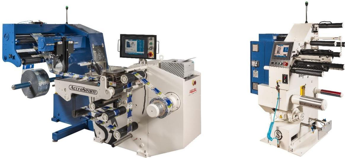
The Stanford AccraSeam™ shrink seamer is the fastest on the market, accurately seaming material while holding industry lay-flat tolerances at 600 MPM (2,000 FPM). Equipped with fully-automated lay-flat adjustment, servo-based tool positioning, and lay-flat monitoring with full reporting, the AccraSeam™ sets a new standard in shrink sleeve converting.
